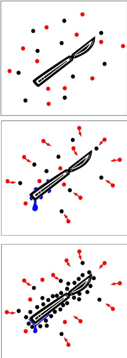
Figure 5 – Steam pushes NCGs toward the instrument surface
