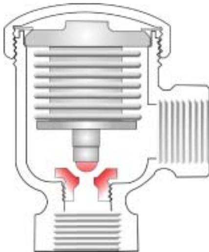
Figure 5: Thermostatic Trap
